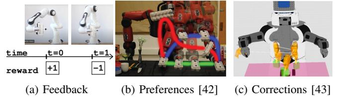
Fig. 4: Teaching with reward (4a), preferences (4b), and corrections (4c). With reward (4a), the person observes the robot and rewards it for past actions, e.g., with a  $\pm 1$  signal. With preferences (4b), the person selects between two or more candidate trajectories; the example in 4b structurally aligns three trajectories, supporting difference detection. Finally, with corrections (4c), a person modifies past trajectories—either through a GUI [43], [44] or physical manipulation [45], [46].
